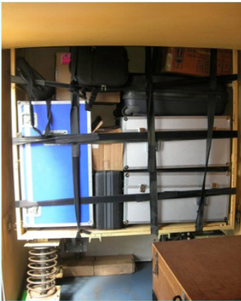
Figure 2: An example of the cases used to protect equipment and the spring shock absorbers used beneath the platforms holding the cases. (Both images courtesy of Krishna Murthy, M.D, Subbakrishna Rao and Prabha Eye Clinic, Bangalore, India.)
